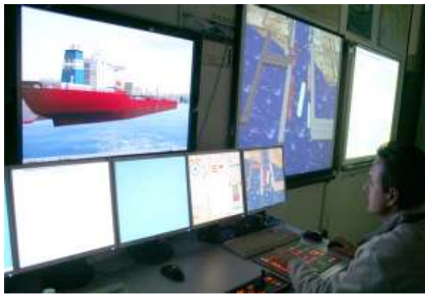
Figure 10: Virtual bridge and active board for guided survey of simulations [6].
